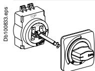
**Extended rotary handle (for 3/4P breaker)**
