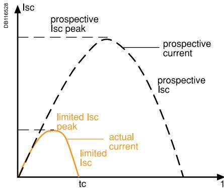
The exceptional limiting capacity of the EasyPact EZC range greatly reduces the forces created by fault currents in devices.
