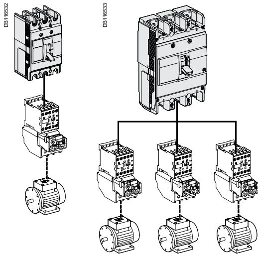
A circuit supplying a motor may include one, two, three or four switchgear or controlgear devices fulfilling one or more functions.
