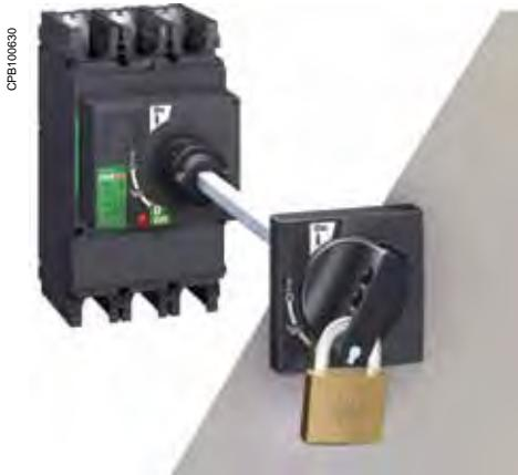
Escutcheons are an optional feature mounted on the switchboard door. They increase the degree of protection to IP40, IK07. Protection collars maintain the degree of protection, whatever the position of the device (connected, disconnected).
