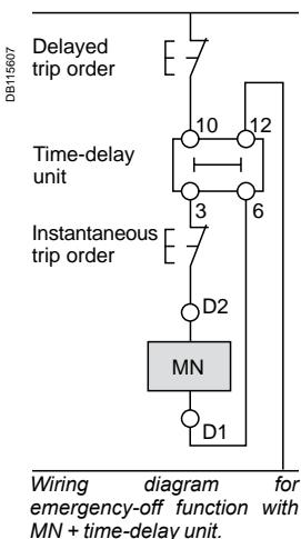
Wiring diagram for emergency-off function with MN + time-delay unit.
