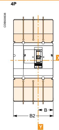
Long terminal shields also available for EZC400/630 spreaders with 52.5 mm pitch:
