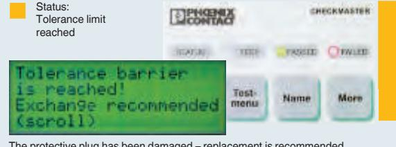
The protective plug has been damaged – replacement is recommended.
