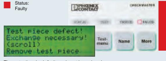
The protective plug is faulty and must be replaced.
